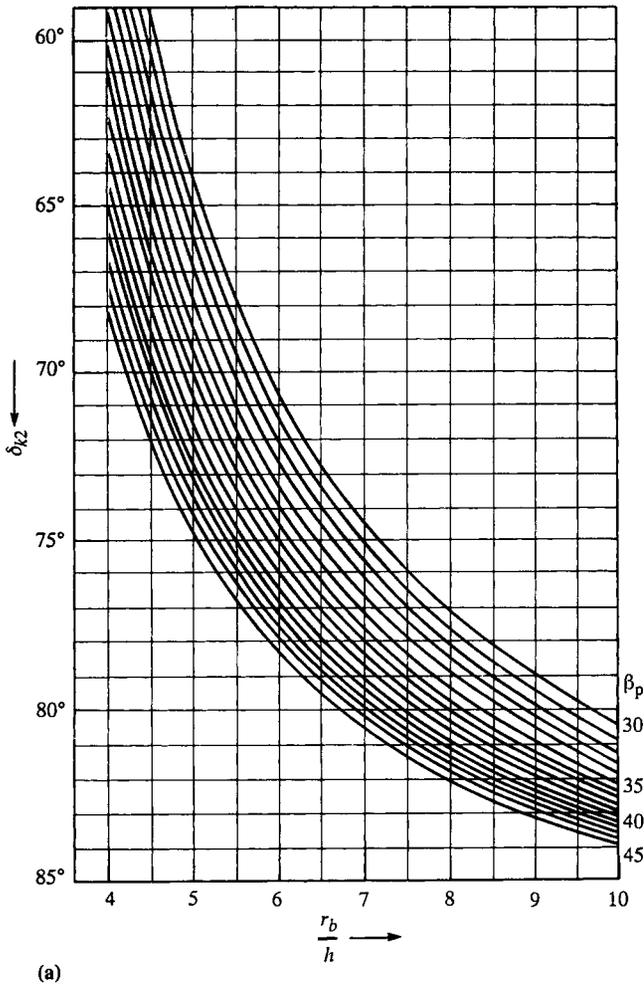
Figure 6.6(a-c) Graphs for cutter spindle tilt: (a)  $C=0^\circ$ ; (b)  $C=1^\circ 30'$ ; (c)  $C=3^\circ$
