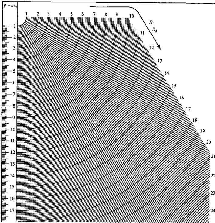
**Figure 5.2(a)** Graph for checking the position of the gear hob – see also Figures 5.2(b) and 5.2(c). If the positions of gear hobs are to be checked which have a cone distance  $R_A$  not given in the graph above, then the positions must be found by drawing them out on millimetre graph paper (Figures 5.2(a), (b) and (c) should be enlarged to 200% their present size for accurate measurement in mm)
