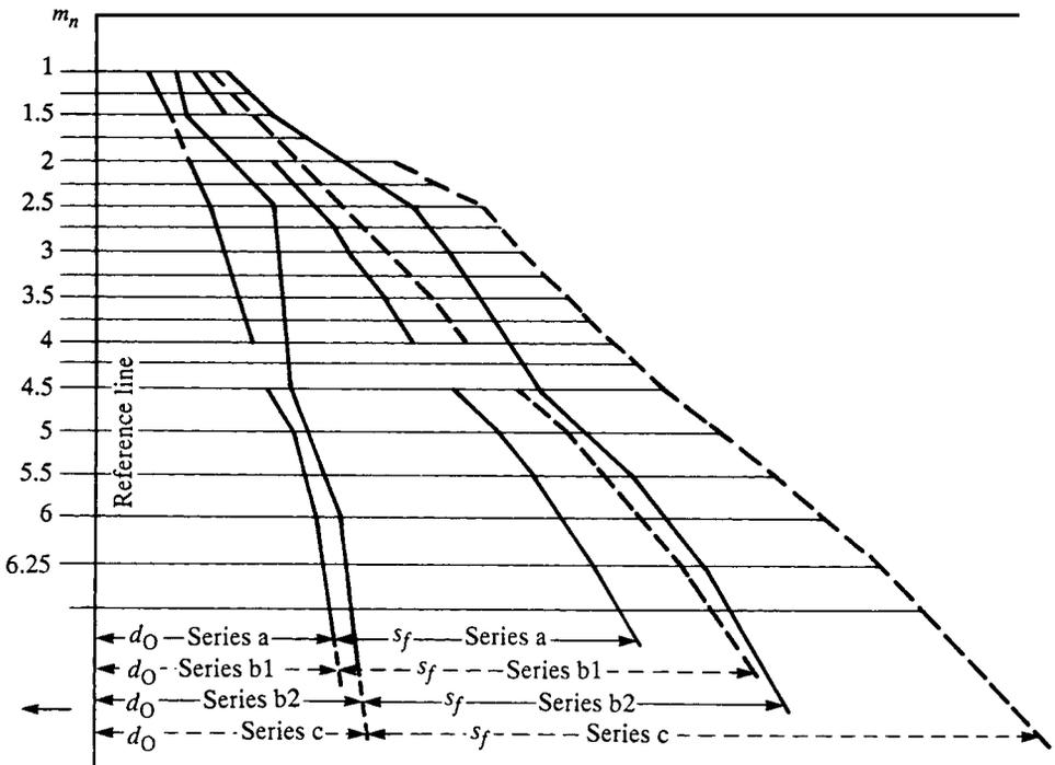
**Figure 5.2(c)** Graph for checking the position of the gear hob – see also Figures 5.2(a) and 5.2(b)
