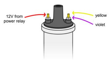
Both ignition outputs from the ECU go onto the coil negative terminal. The distributor can be left as standard but all that is now used are the rotor arm and cap; the advance mechanisms, points etc are redundant.
