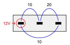
Some valves have the diodes inbuilt and will have a diode diagram on them. If so, the polarity of the wiring must be as shown below.
