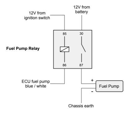
The power supply relay for the injectors, coil, lambda sensor etc is also controlled by the fuel pump output.
