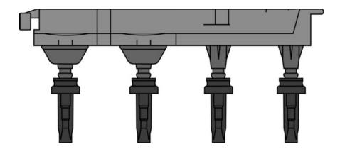
The coil should be non-amplified. You can test this by measuring with a multimeter (resistance setting). Between the 12V terminal and one of the signal terminals (also known as coil negative) a non-amplified coil will measure approximately  $1\Omega$ . An amplified coil pack will measure several  $k\Omega$ . Amplified coil packs can be used if necessary, but are not ideal and the ECU hardware must be modified by Omex to allow this.
