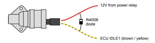
The diode in the wiring is required. The polarity of the wiring onto the valve is not important, but the polarity of the diode with respect to the wires is. The marked blocking end must face the 12V wire.
