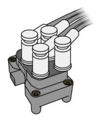
Some engines have wasted spark coil packs that look like 4 individual coils, but are still two double ended coils and so can still be controlled directly by the ECU. Examples are some Rover K Series and some small Peugeot engines;
